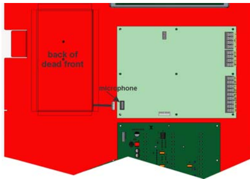
Figure 7: Microphone Cord Inserted Through Dead Front Panel Hole
