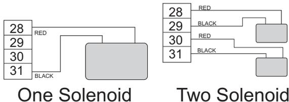
Figure 5. Release circuit used to fire solenoid control head(s), P/N 48650001 or 899175. Wiring polarity must be as shown for P/N 48650001. P/N 899175 is non-polarized.
