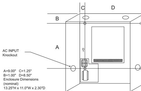
Figure 2. Mounting Dimensions
